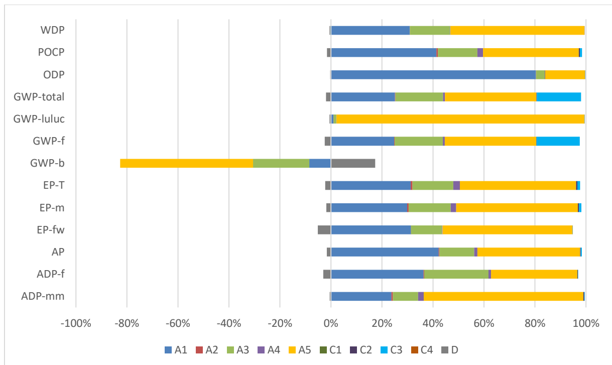
Figure 1: Dr. Schutz® PU Anticolor - Impact of the individual modules on the environmental core indicators
