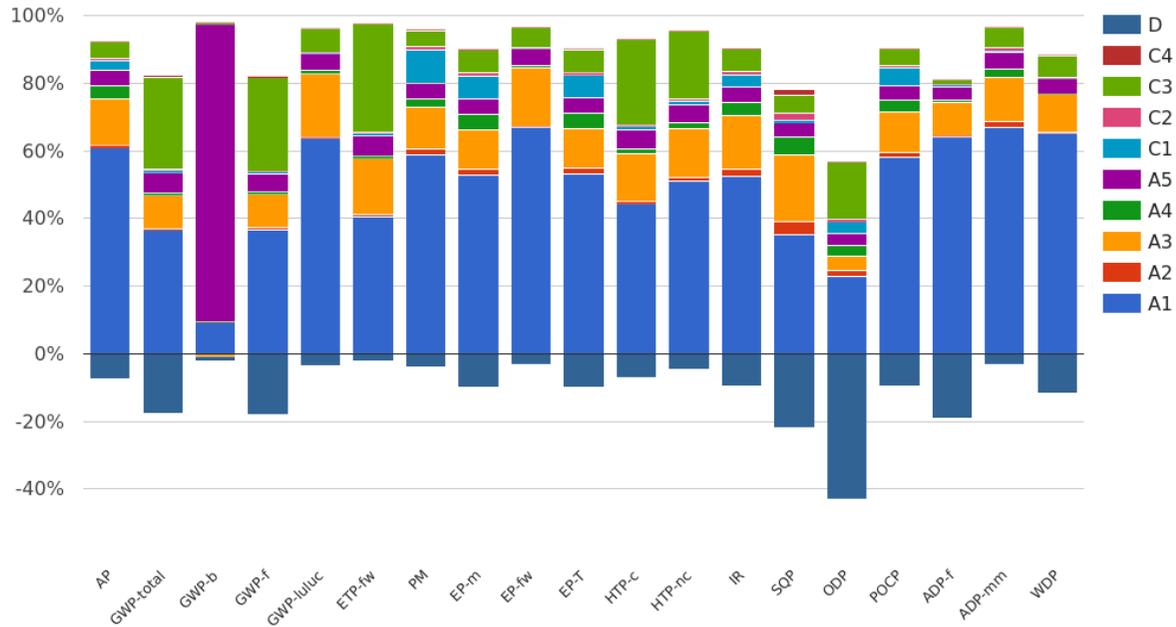
As shown in the figure below, the raw material supply (A1) dominates in most environmental core indicators, followed by production process (A3). The highest influence on the Global Warming Potential (GWP-total) have raw material supply (A1) and waste processing (C3).
