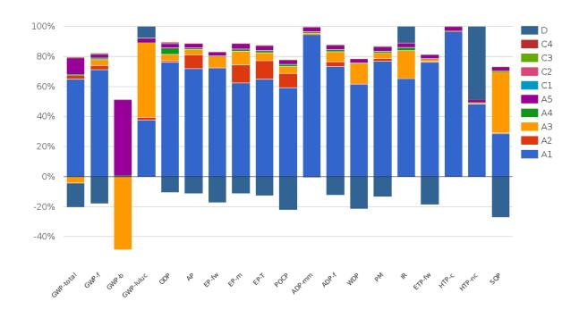
The figure shows the influence of the different life stages on the environmental core indicators for the clothing rack. As shown in the figure the majority of the environmental impacts are attributed to the raw material processing phase (Al) and the production process (A3). The benefits and loads beyond the system boundary (D) have a considerable impact across most of the environmental impact categories.
